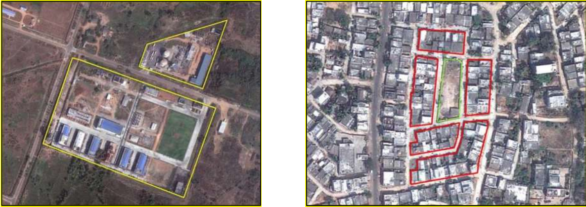
Figure 5-2 GCPs for DGPS Survey marked on Satellite Imagery
