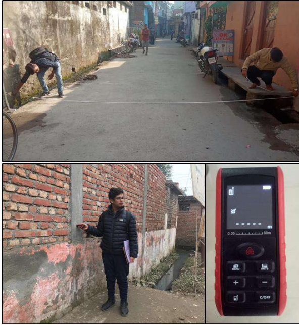
Figure 5-4 Sample Road Inventory by using Laser Distance Meter
